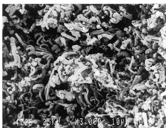
Fig. 4. Carbon filaments and amorphous carbon. (from [39]).
